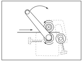
Figure 17. Flat rolling the workpiece.
